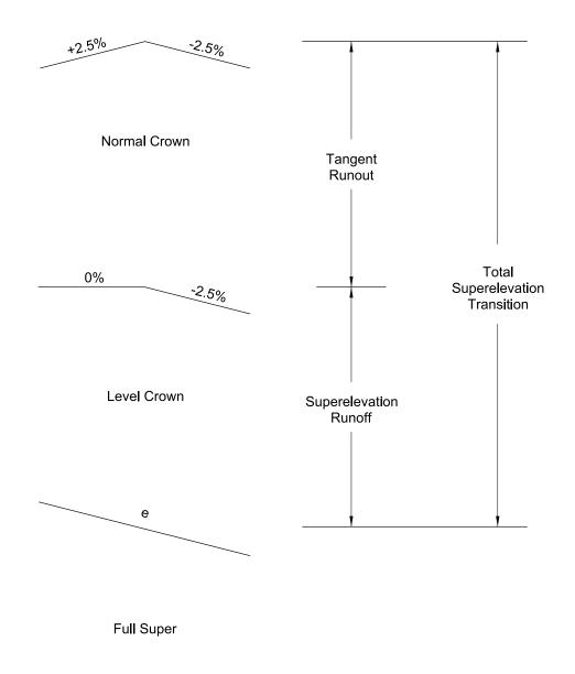
e = Full Superelevation Rate
